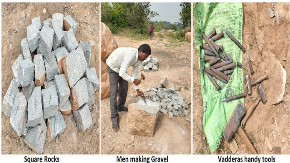
Fig 5.3: Square stone blocks (made by men); gravel making by men; basic tools of stonework
